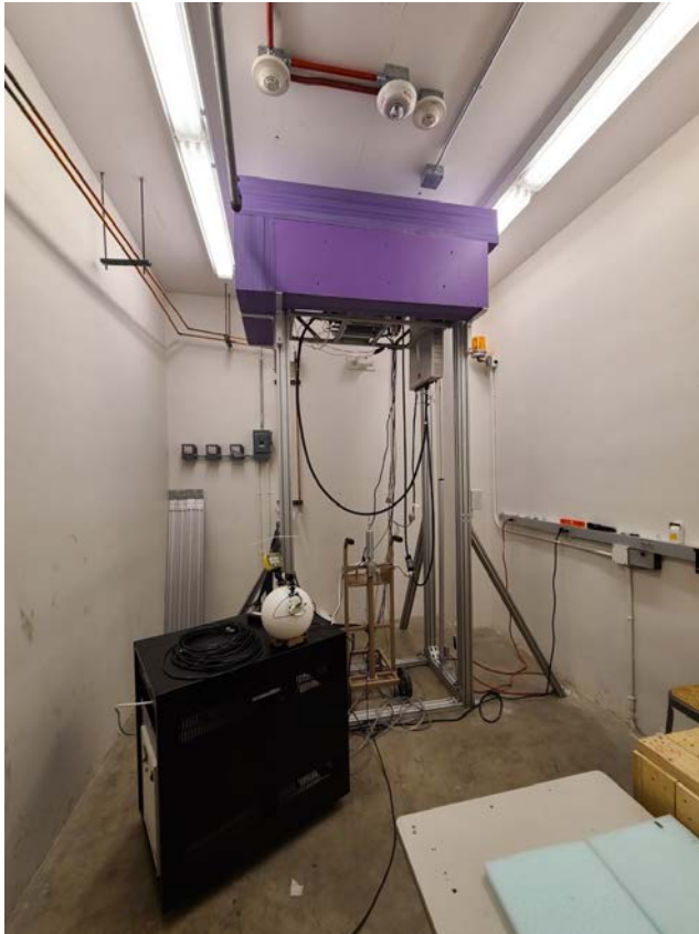
a) Thermal neutron detector in beamline
